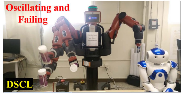
Fig. 2. The robot fails to track the desired trajectory without a predictor in the presence of input delay.
