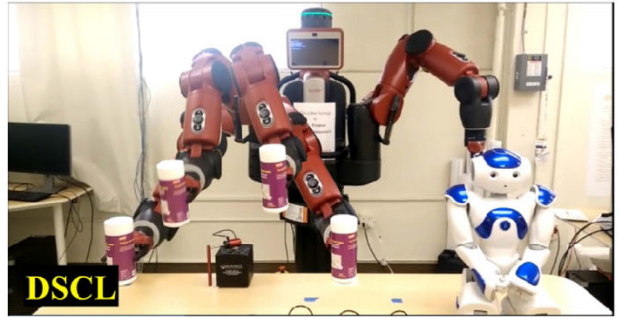
Fig. 3. A stable obstacle-avoidance pick-and-place task with input delay using the predictor-based controller.
