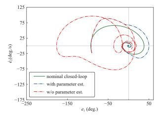
Fig. 5. The projection on the  $e_1$  vs.  $\dot{e}_1$  plane solution of the closed-loop system with the proposed controller.
