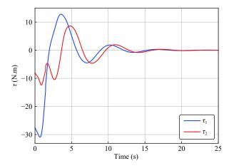
Fig. 4. The control torques of the joints in the case of having parameter estimation update.
