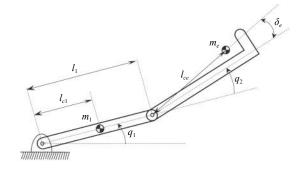
Fig. 1. A two-link manipulator.
