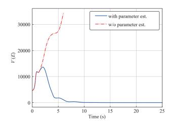
Fig. 7. The values of Lyapunov function for the closed-loop system with the proposed controller.
